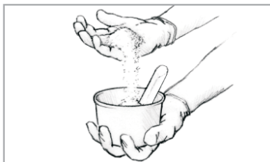
Figure 5 Stir in small handfuls of filler until the desired consistency is reached.
