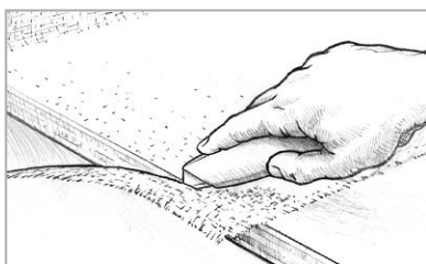
Figure 26 Trim excess cloth after the epoxy gels.
