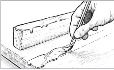
Figure 9 Apply resin/hardener mixture to the bonding surfaces.
