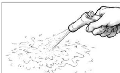
Figure 33 Rinse the surface with fresh water after sanding.
